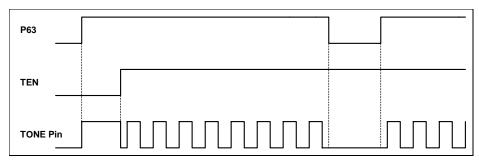
Fig. 5-7 Tone Output Pin Timing Chart
